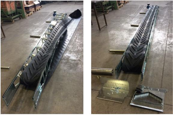
8 – Refit the tension cylinder, the return rollers and the tension plates.
