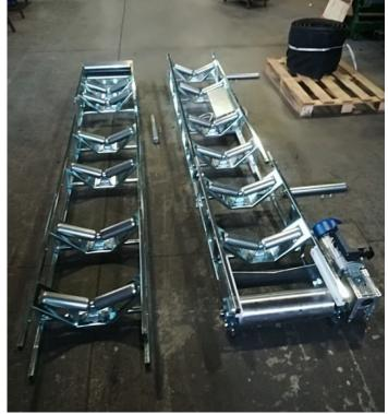
2 – Mount the intermediate frame with the control frame, first remove the return roller from the support bracket
