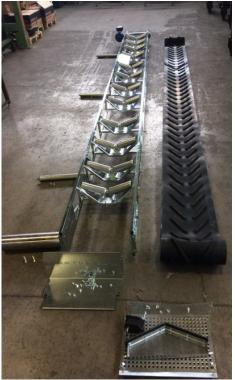
7 – Insert the rubber belt on the tension and then on the control
