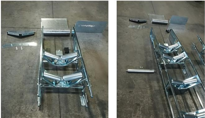
5 – Mount the intermediate frame with the tension frame and tighten the joints firmly
